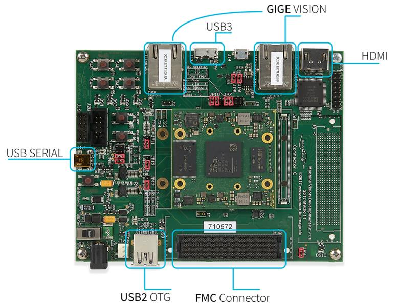
*Sensor to Image MVDK (Machine Vision Development Kit) is a hardware platform that eases the evaluation and development of products based on S2I's IP Cores and using any major industrial vision interface. The MVDK base board is highly configurable through the use of FMCs (FPGA Mezzanine Cards). It provides an interface to vision sensors and enables the development of GigE Vision, USB3 Vision and CoaXPress cameras (devices), as well as the design of GigE Vision and CoaXPress hosts.*
